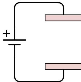
Figure 8 - Circuit diagram of DC high voltage supply and aluminum electrodes at either end of chamber (in pink). This circuit was used for prototyping before the circuit in Fig. 9 was built and implemented.
