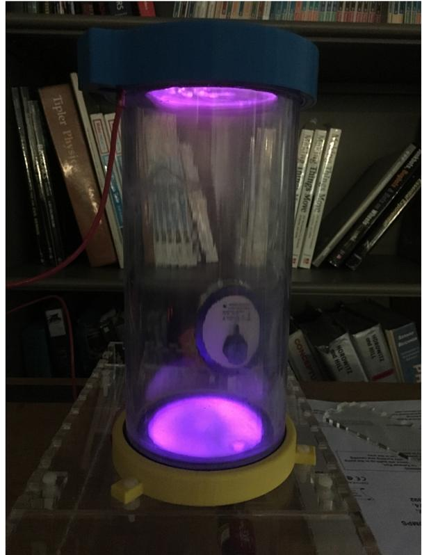
Figure 12 - Glow plasma clinging to the electrodes at extremely low pressure
