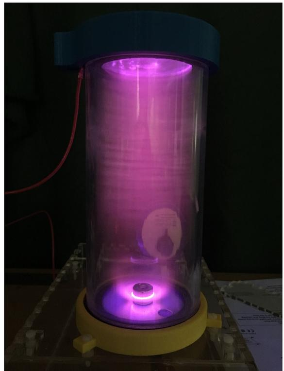
Figure 17 - Torus Magnet with Band at Lower Pressure than Fig. 15
