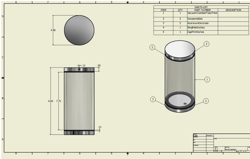
Figure 5 - CAD drawing of chamber with aluminum disks, neoprene seal, and acrylic cylinder
