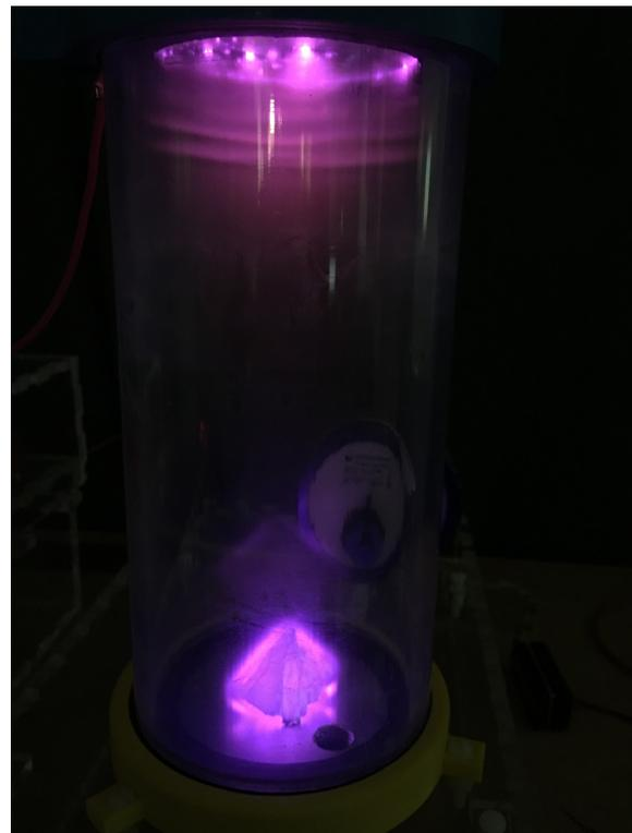
Figure 19 - Pointed Aluminum Foil Electrode at Very Low Pressure
