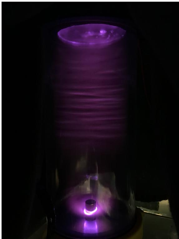
Figure 16 - Double Cylinder Magnet with Plasma Band and Wave Effect
