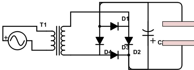
Figure 9 - Circuit diagram of line power supply running through a transformer to step up voltage, and a rectifier and capacitor to convert AC to DC. This setup was used with the final chamber because the circuit in Figure 8 did not provide enough voltage to generate plasma with the electrode spacing used for the chamber.
