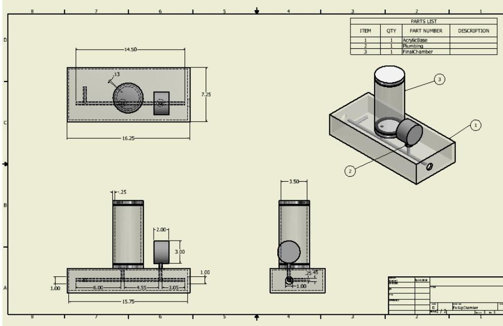
Figure 6 - CAD drawing of chamber including acrylic base and plumbing. Does not include plastic end caps (see Fig. 7).
