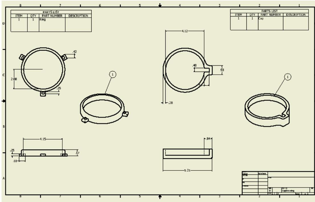
Figure 7 - CAD drawing of 3D printed protective ring for bottom electrode (left) and 3D printed protective cap for top electrode (right).
