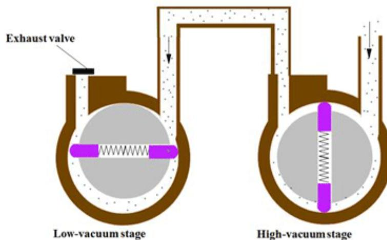
Figure 4 - Diagram of two stage rotary vane pump (Edwards Vacuum via Vac Aero International)
