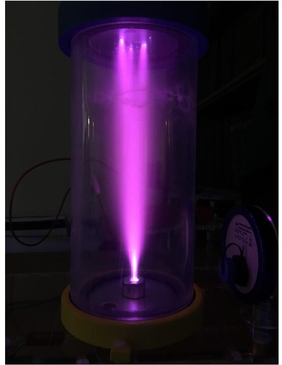
Figure 15 - Plasma Jet from Upright Torus Magnet
