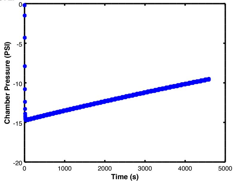
Plot 1 displays the data from a test of the vacuum pump's effectiveness in conjunction with the chamber. From these data, it takes the vacuum pump between 20 and 30 seconds to reach the chamber's minimum pressure. Plot 2 displays data from the same test as Plot 1, but it includes the pressure in the chamber for 1 hour, 16 minutes, and 30 seconds after the vacuum pump is
