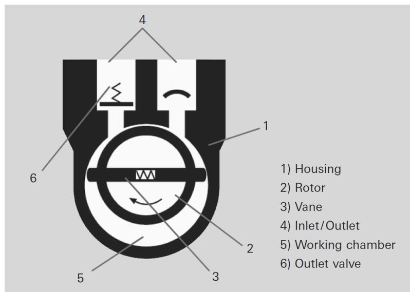
Figure 3 - Diagram of pumping apparatus in a rotary vane pump (Pfeiffer Vacuum)
