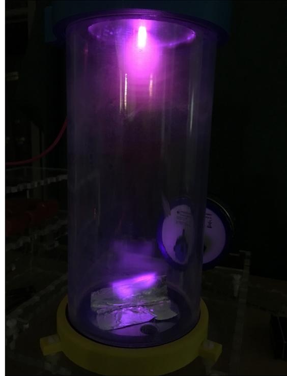
Figure 21 - Pointed Ridge Aluminum Electrode
