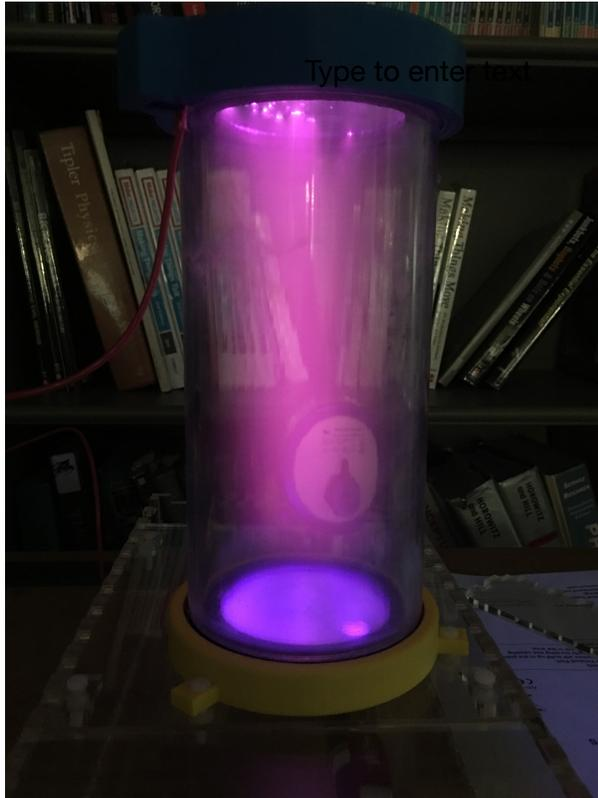
Figure 11 - Stable glow plasma filling the chamber at around 300Pa
