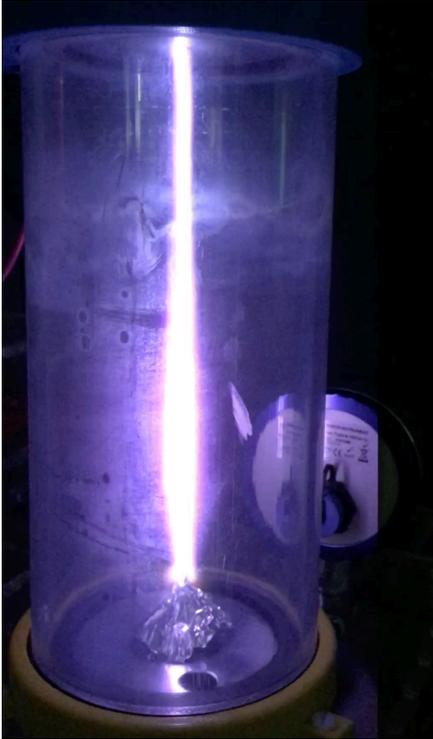
Figure 20 - Arcing at Higher Pressure To Pointed Aluminum Foil
