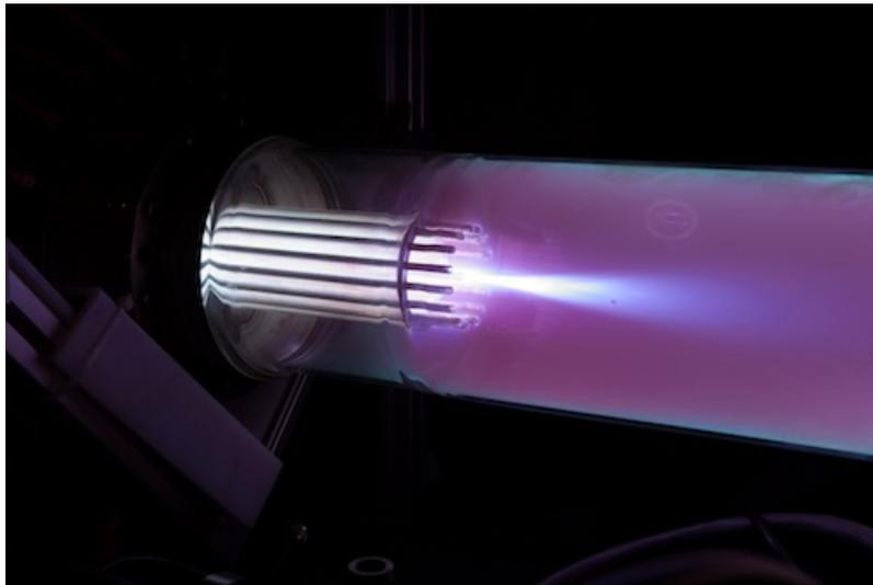
Figure 1 - "The Stanford CHENG Gun (SCG) is a pulsed, direct electrode plasma source that produces a high velocity, high energy density plasma jet in vacuum." (Stanford Plasma Physics)
