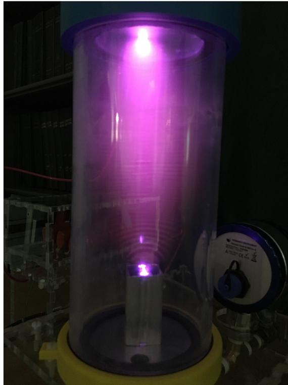
Figure 23 - Aluminum Bar Electrode with Small Central Gap
