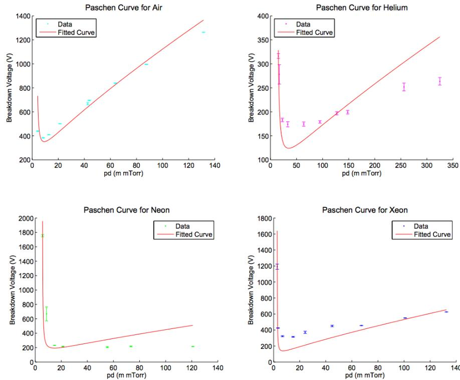
Figure 10 - Empirically determined Paschen's curves for Air, Helium, Xenon, and Neon (Paschen's Law in Air and Noble Gases, Berzak, et al.)
